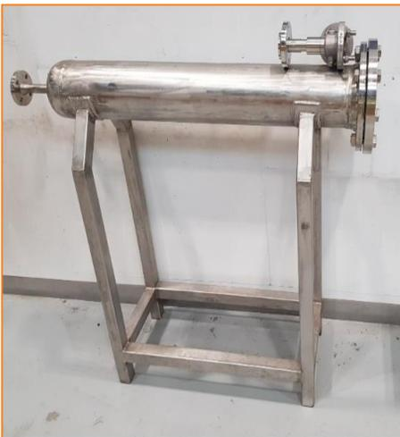
The second and third tests use specialized equipment to increase and alter the type of corrosion induced on the samples. The second test uses geothermal steam that has been separated within the geothermal plant. The steam is fed into a pressure vessel which holds the samples and oxygen is added into the vessel to increase the corrosive effects and to simulate the axial seal system suction path where corrosion is pervasive in many geothermal plants.
