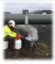
The analysis has revealed a substantial concentration in  $\mathrm{CO_2}$  and  $\mathrm{H_2S}$ , together with a high temperature of the geothermal fluid. Results from the analysis will help defining the experimental conditions for the lab-testing of the coatings in the project. Results will be made available to the public.
