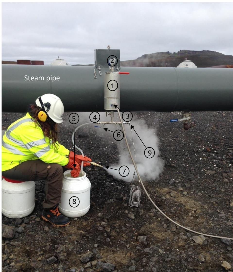
**Figure 4:** Setup when sampling for steam. Numbers on figure correspond to numbers in the method above (photo: Sigrún Sif Sigurðardóttir).
