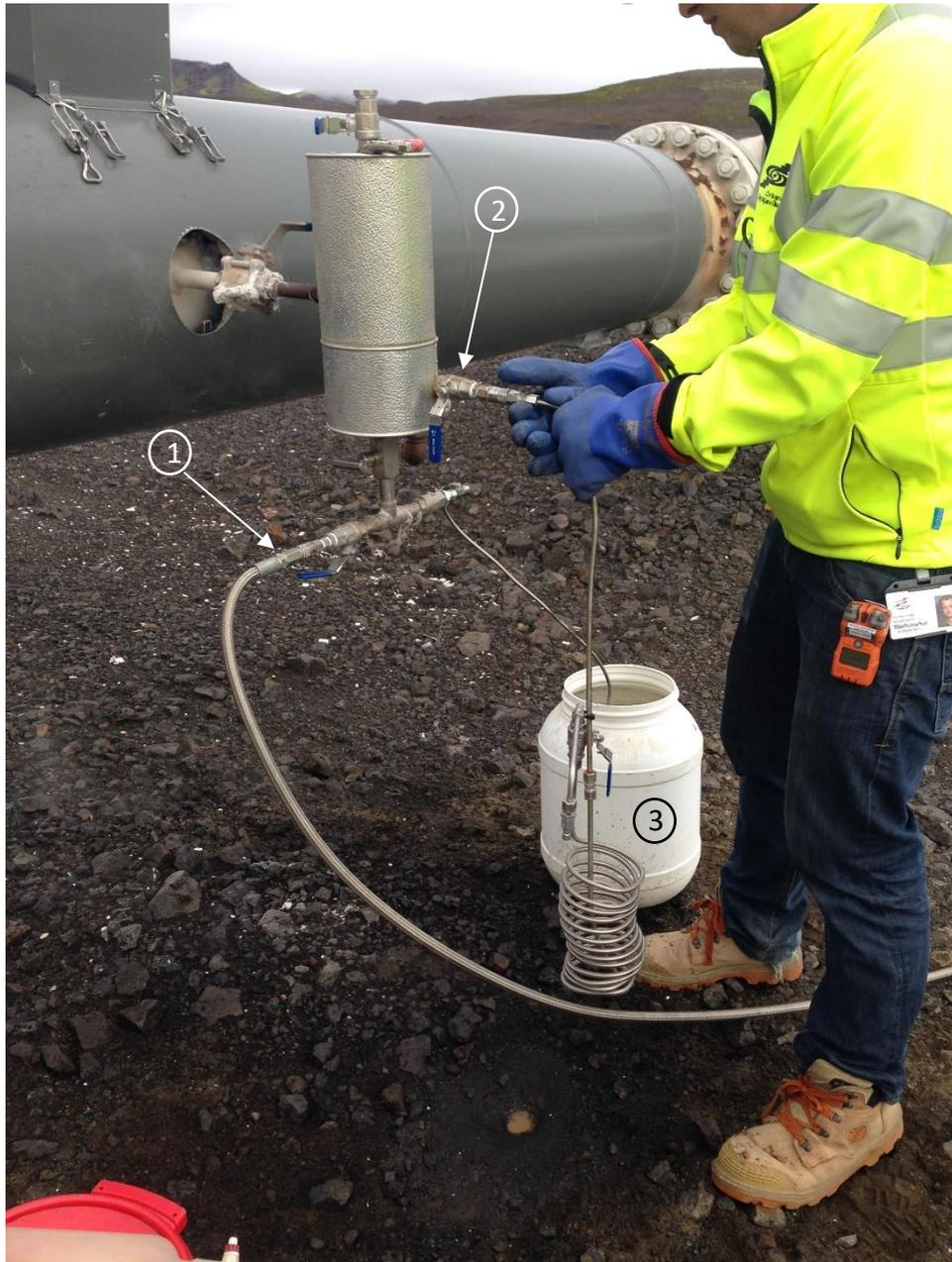
*Figure 5: Setup when sampling for water. Numbers in figure corresponds to numbers in the method (photo: Sigrún Sif Sigurðardóttir).*
