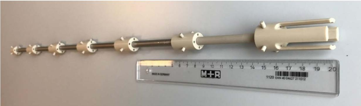
**Figure 4: Actual components of the PEEK sample holders assembled with carbon steel rod samples for demonstration purpose.**
