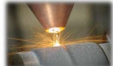
Laser Metal Deposition (LMD) process
