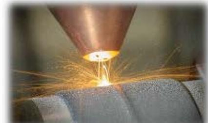
Laser Metal Deposition (LMD) process
