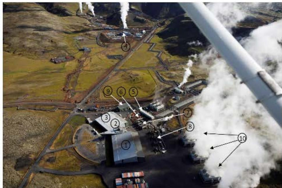
Figure 1: Overview of Hellisheiði power plant. 1) Turbines 1-4, 2) turbine 11, 3) heat exchanger, 4) turbines 5 and 6, 5) main building for fluid distribution, 6) boiler, 7) low pressure separators, 8) moisture separators, 9) workshop, 10) cooling towers (photo: Gretar Ivarsson).
