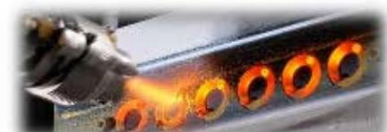
High-Velocity Oxygen Fuel (HVOF) process
